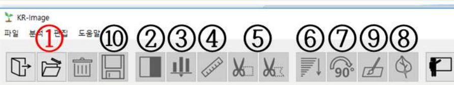
① Open file → ② Binarization → ③ Noise filtering(noise) →
