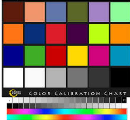
10. The light source is of large influence on the observed color in the image. Especially for color, the type of light source is important. In many cases, lamp color and intensity change during warming up of the lamps, so let them burn about 15 minutes before starting the recordings. If fluorescent tubes are used, check regularly if they still have more or less the same intensity/color, as they may change rather rapidly with age. You can use the calibration chart for notification.
