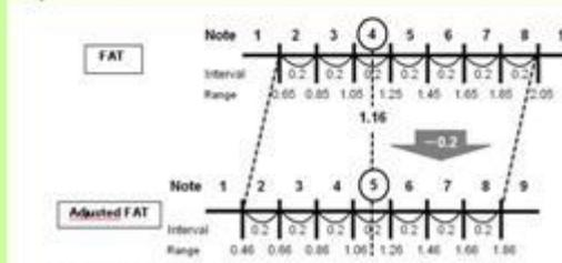
Fig. 3 Adjustment FAT with the sliding method
