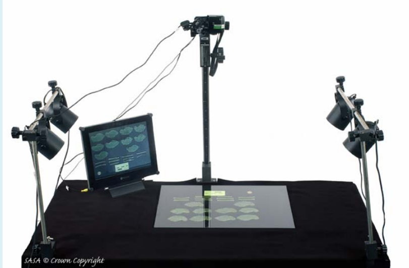
SASA © Crown Copyright Canon EOS 450D digital camera linked to computer; IMAGIN programme; lens EF-S 18-55 IS Kit. Camera is 64 cms above plant parts. 4 x 11W energy saving light bulbs (ES/E27 Screw Cap). Pea leaflets and stipules are flattened by acrylic sheet.
