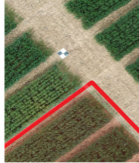
Detail image with ground control point (GCP)
