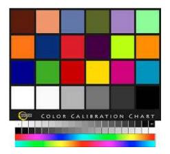
9. 40. The light source is of large influence on the observed color in the image. Especially for color, the type of light source is important. In many cases, lamp color and intensity change during warming up of the lamps, so let them burn about 15 minutes before starting the recordings. If fluorescent tubes are used, check regularly if they still have more or less the same intensity/color, as they may change rather rapidly with age. You can use the calibration chart for notification.
