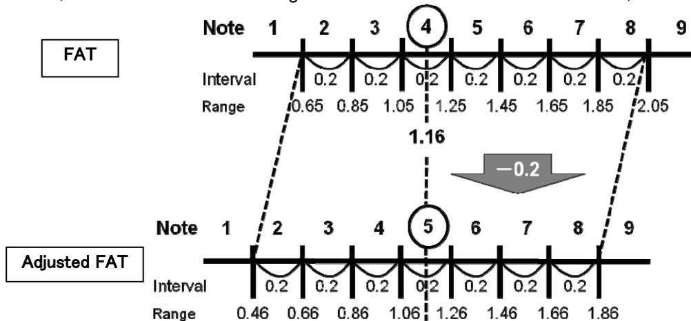
Fig.3: Adjustment FAT with the sliding method
