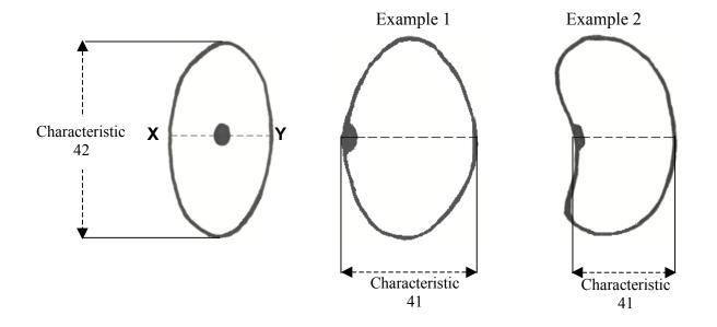
Characteristic 40: shape in cross section (**X-Y** = cross section)
