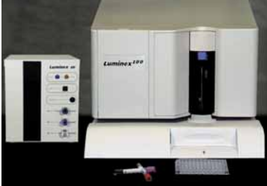
Fig. 9 Luminex® Apparatus for High-Speed throughput Analysis using Immunobeads (Source: Luminex Corporation)
